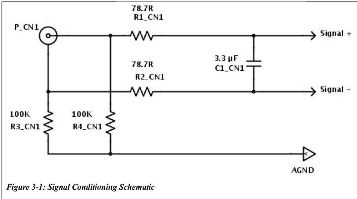
The components R1, R2 and C1 create a passive low-pass filter. The corner frequency of the filter is approximately 306 Hz. The filter is designed to reduce the energy in the input signal before sampling to reduce aliasing without introducing unwanted attenuation in the frequency range of interest and without adding significant phase lag.
