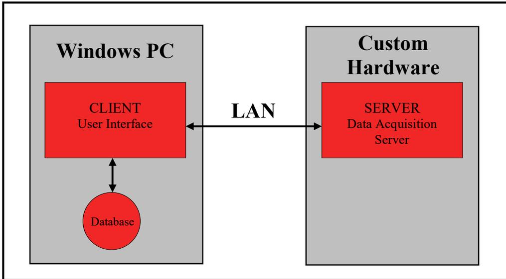
Figure 1-1: ADQ-1000: WaveGen-Studio with Data Acquisition Server
