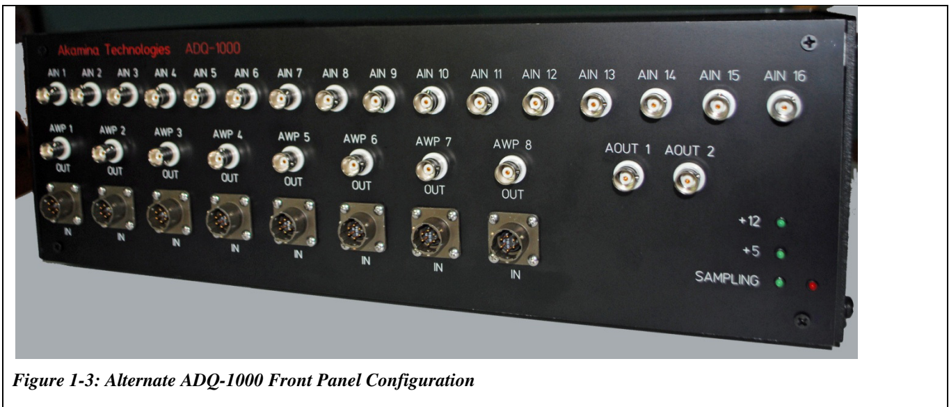
Figure 1-2: ADQ-1000 with 16 Analogue Input Channel Analogue
