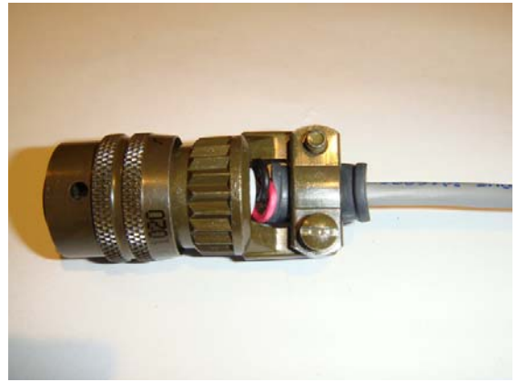
Figure 14: Strain relief completed
